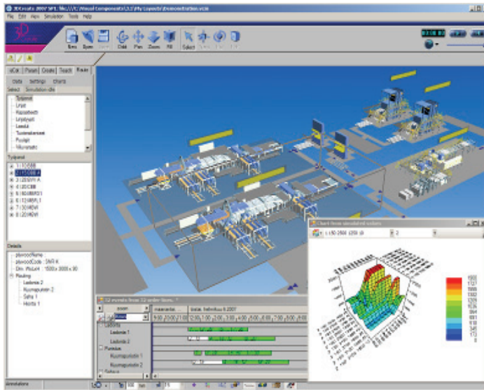
Fig. 11. Raute case simulation, plywood factory with Raute equipments.
