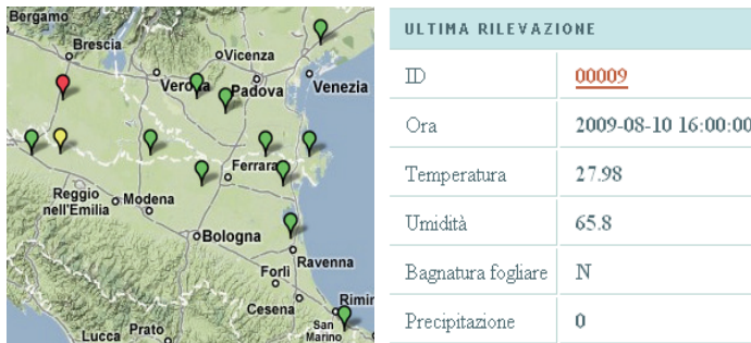
Fig. 9. Example of the DSS tool showing the real-time working status of the agro-meteorological stations. Green markers indicate a regular flux of data, yellow markers signal a short delay of the station in sending data, while red markers indicate that no data are coming from the station. When the user clicks on the proper marker, the table shows the current data measured by any station selected.
